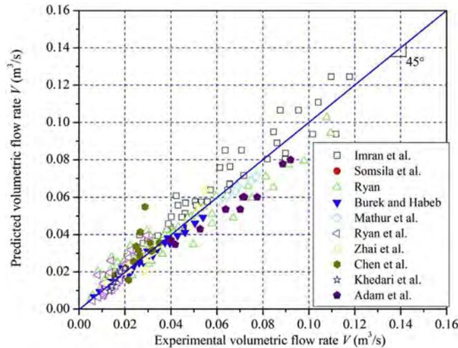
**Fig. 15.** A comparison between experimental and predicted volumetric flow rate by Eq. (19).
