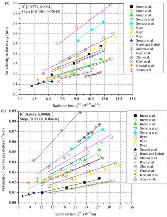
Fig. 12. Correlation between radiation heat and: (a) air velocity in the cavity; and (b) Volumetric flow rate per meter.
