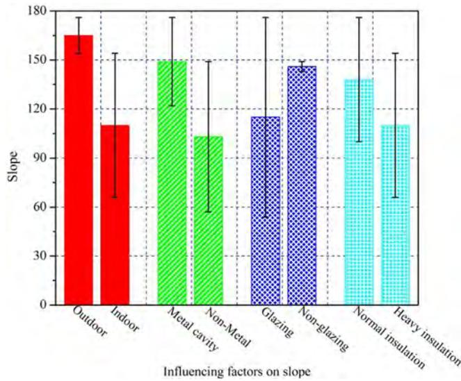
**Fig. 14.** The influencing factors on the slopes obtained from the regression between the experimental airflow rate  $V$  and  $w(\sin\theta')^{1/3}q^{1/2}d^{0.7}H^{2/3}$ ; and a small slope means an enhanced performance of solar chimney.
