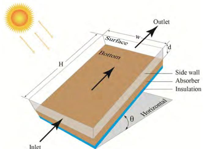
Fig. 1. Schematic of a typical test rig for roof solar chimney.
