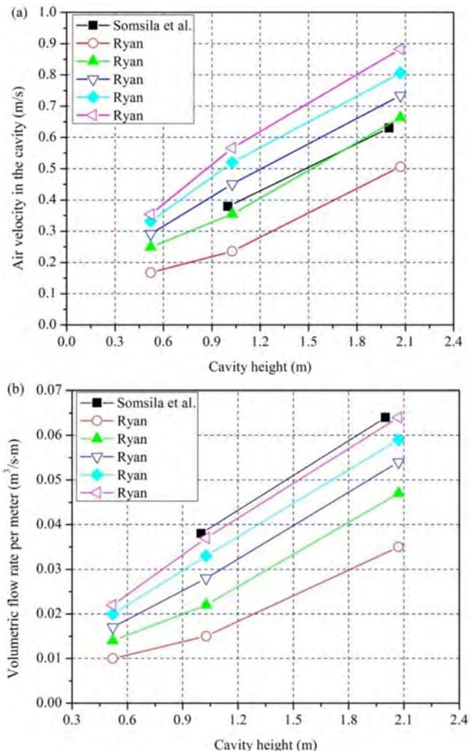
Fig. 6. The influence of cavity height on: (a) air velocity in the cavity; and (d) volumetric flow rate.
