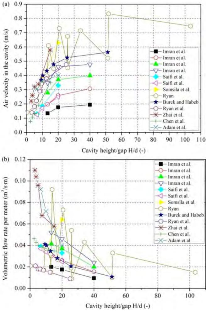
Fig. 9. The influences of cavity height/gap ratio on: (a) air velocity in the cavity; and (b) volumetric flow rate.
