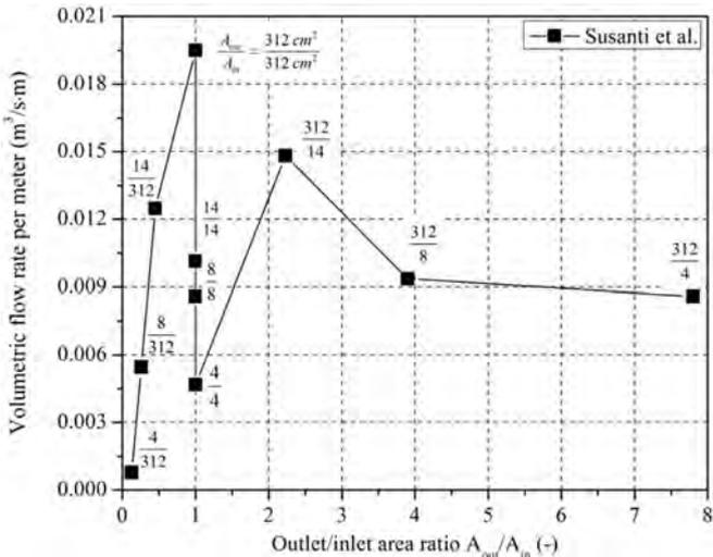
Fig. 10. The influence of outlet/inlet area ratio on volumetric flow rate per meter.
