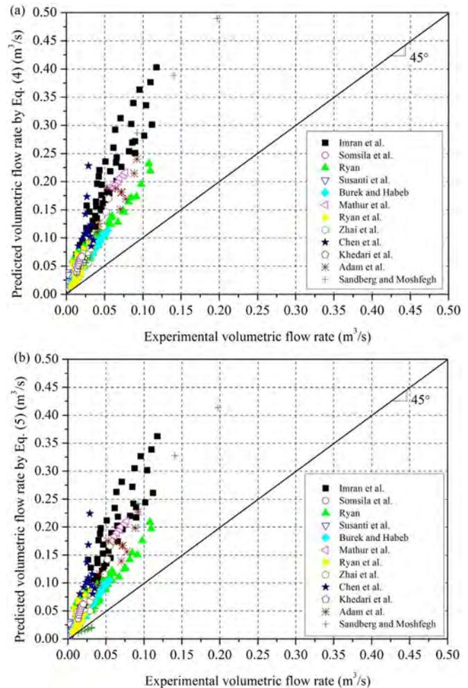
Fig. 2. A comparison between the experimental data and predictions based on: (a) Eq. (4); and (b) Eq. (5).
