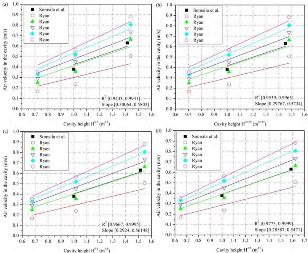
Fig. 7. Correlation between air velocity in the cavity and cavity height: (a)  $H^{0.5}$ ; (b)  $H^{0.539}$ ; (c)  $H^{0.6}$ ; and (d)  $H^{2/3}$ .
