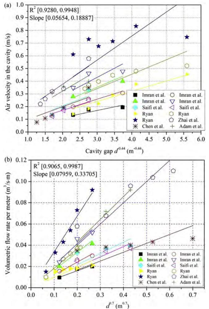
Fig. 5. Correlation between cavity depth and: (a) air velocity in the cavity; and (b) volumetric flow rate per meter.
