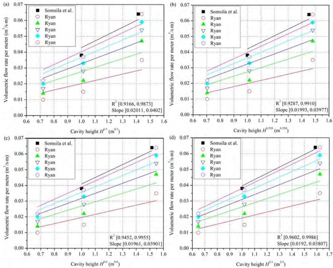
Fig. 8. Correlation between volumetric flow rate and cavity height: (a)  $H^{0.5}$ ; (b)  $H^{0.539}$ ; (c)  $H^{0.6}$ ; and (d)  $H^{2/3}$ .
