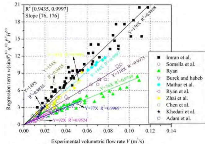
Fig. 13. Correlation between experimental volumetric flow rate and influencing factors.
