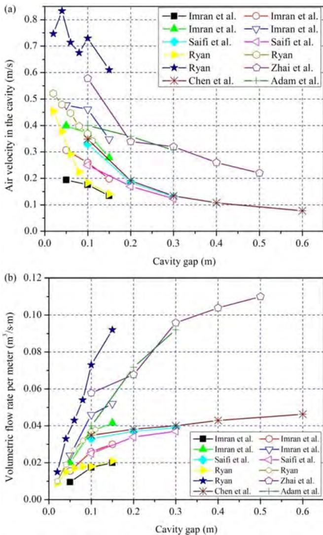
Fig. 4. The influence of cavity gap on: (a) air velocity; and (b) volumetric flow rate.
