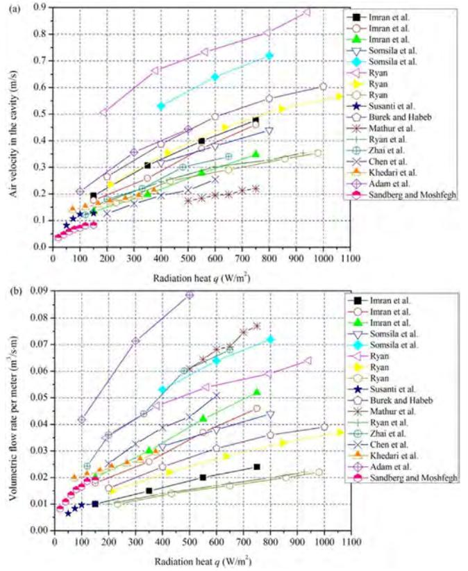
Fig. 11. The influence of radiation heat on: (a) air velocity in the cavity; and (b) volumetric flow rate per meter.
