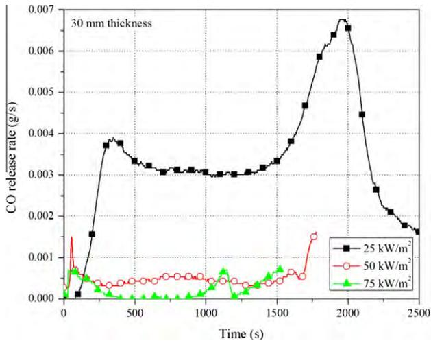
Fig. 6. CO release rate of beech dependent on external heat flux.
