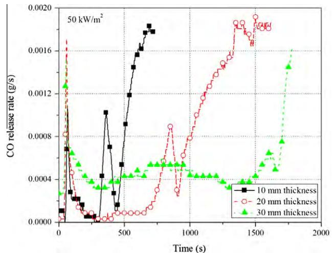
Fig. 4. CO release rate of beech dependent on thickness under  $50 \text{ kW/m}^2$  external heat flux.
