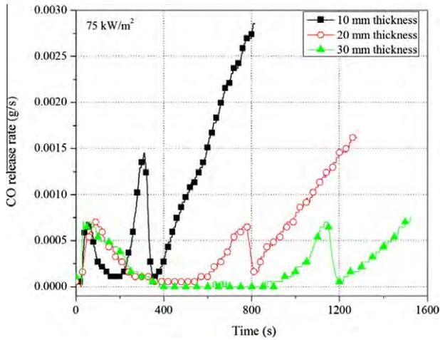
Fig. 5. CO release rate of beech dependent on thickness under 75 kW/m<sup>2</sup> external heat flux.
