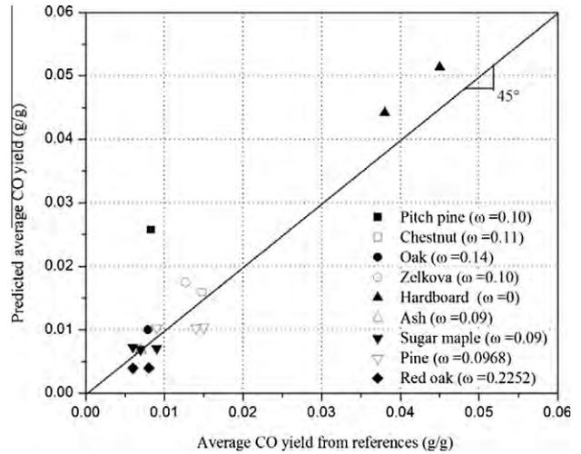
Fig. 14. Comparison between predicted CO yield and reference data.
