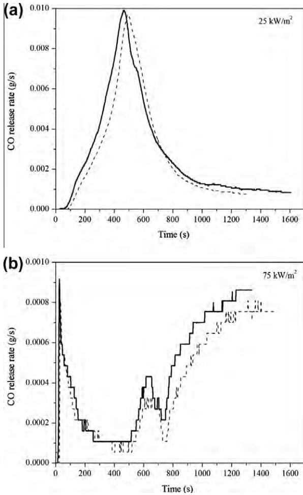
Fig. 2. Repeatability of experiments is good: (a) 10 mm thickness dry wood; and (b) 20 mm thickness wet wood.
