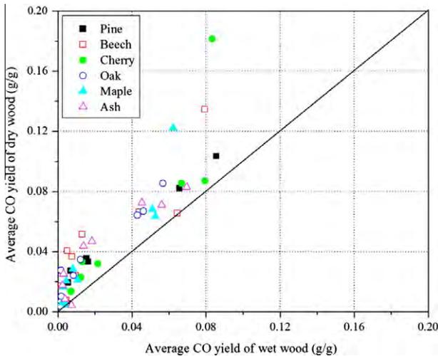
Fig. 12. A comparison of average CO yield between wet wood and dry wood.
