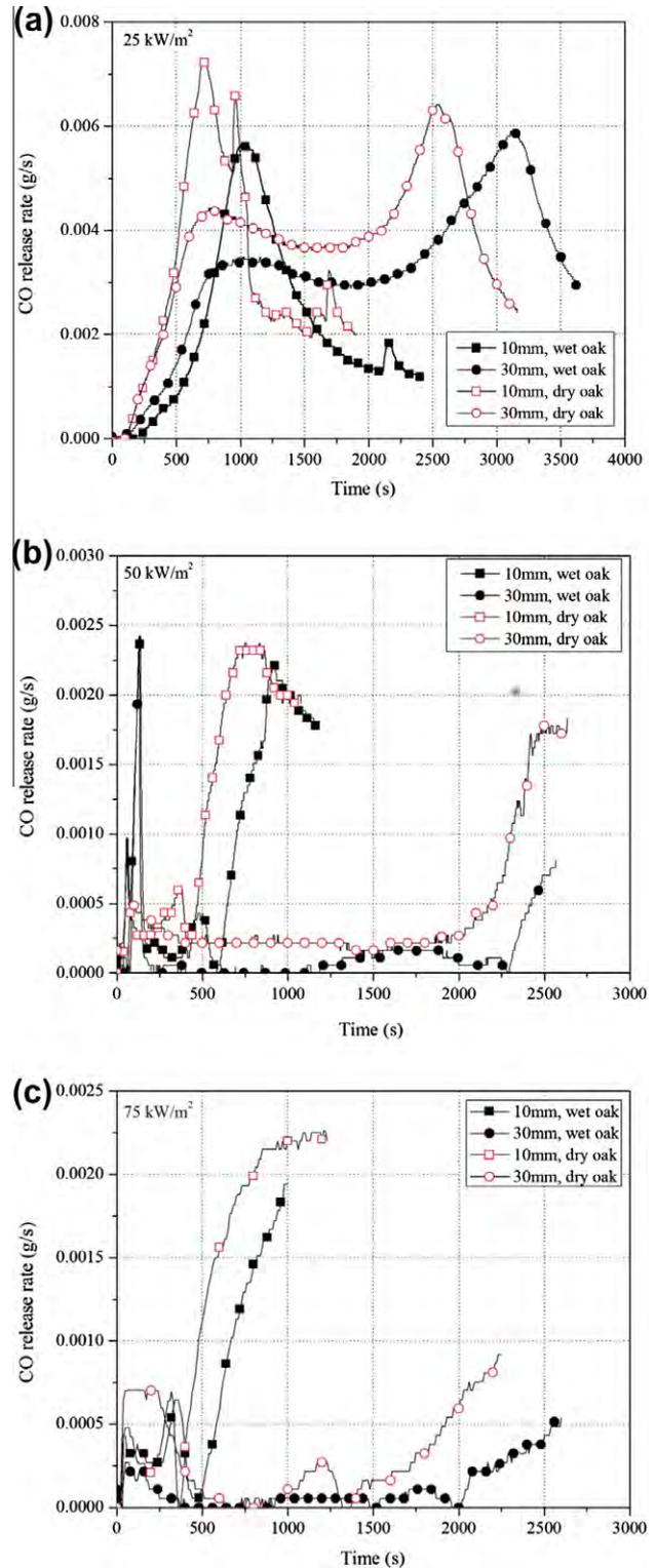
Fig. 11. CO release rate of wet and dry oak under external heat flux (a) 25 kW/m<sup>2</sup>; (b) 50 kW/m<sup>2</sup>; and (c) 75 kW/m<sup>2</sup>.
