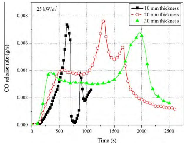
Fig. 3. CO release rate of beech dependent on thickness under  $25 \text{ kW/m}^2$  external heat flux.
