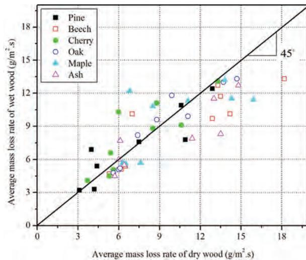
**Figure 8.** Comparison of average mass loss rate between dry wood and wet wood.
