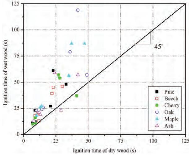
Figure 4. Comparison of ignition time between dry wood and wet wood samples.
