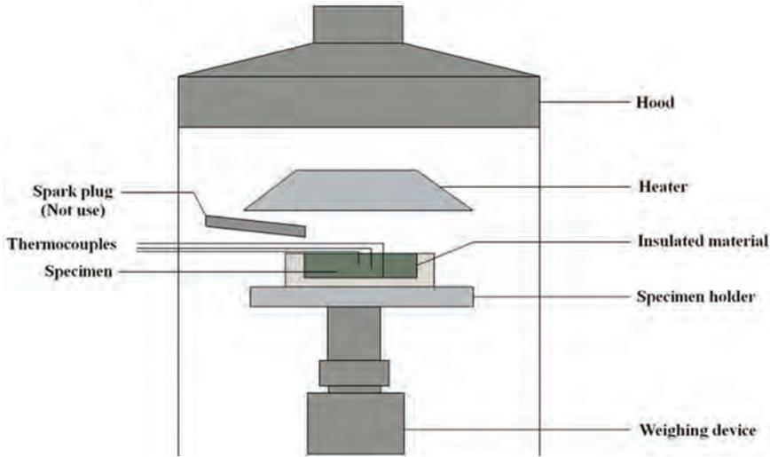
**Figure 1.** The view of wood sample in cone calorimeter.
