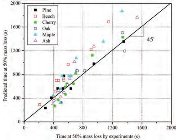
**Figure 10.** Comparison of time at 50% mass loss between experimental data and prediction.
