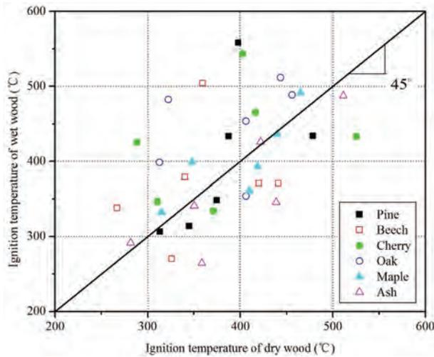
**Figure 2.** Comparison of ignition temperature between dry wood and wet wood.
