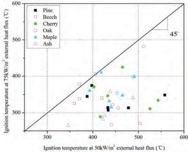
**Figure 3.** The influence of external heat flux to ignition temperature.
