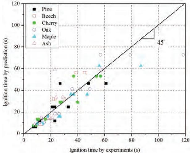
**Figure 7.** Comparison of ignition time between prediction and experiments.
