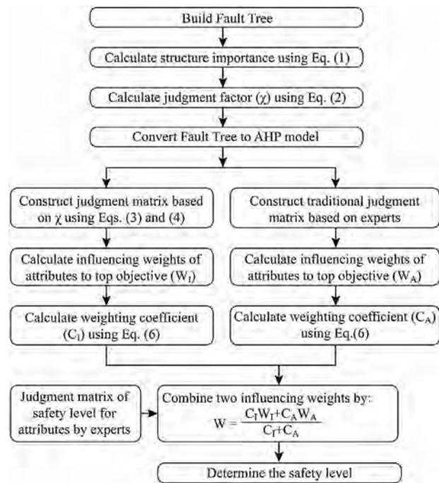
Fig. 1 – The calculation procedure of IAHP.
