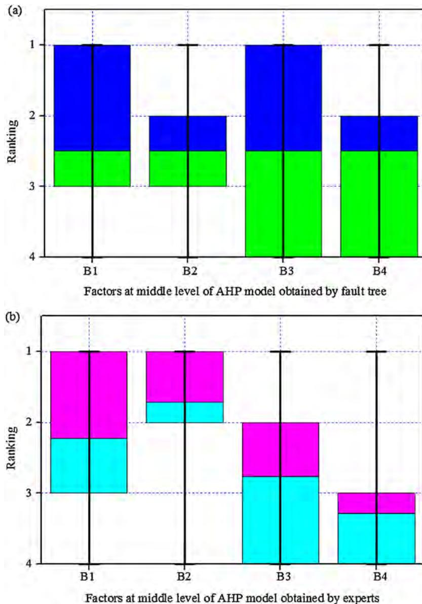
Fig. 4 – Sensitivity analysis of the middle level of AHP models obtained by fault tree (a) and experts (b). The upper and lower caps show their best and worse rankings, while the horizontal lines inside the box are their average rankings, and the upper and lower sides of the box show the 25% and 75% of the ranking results.
