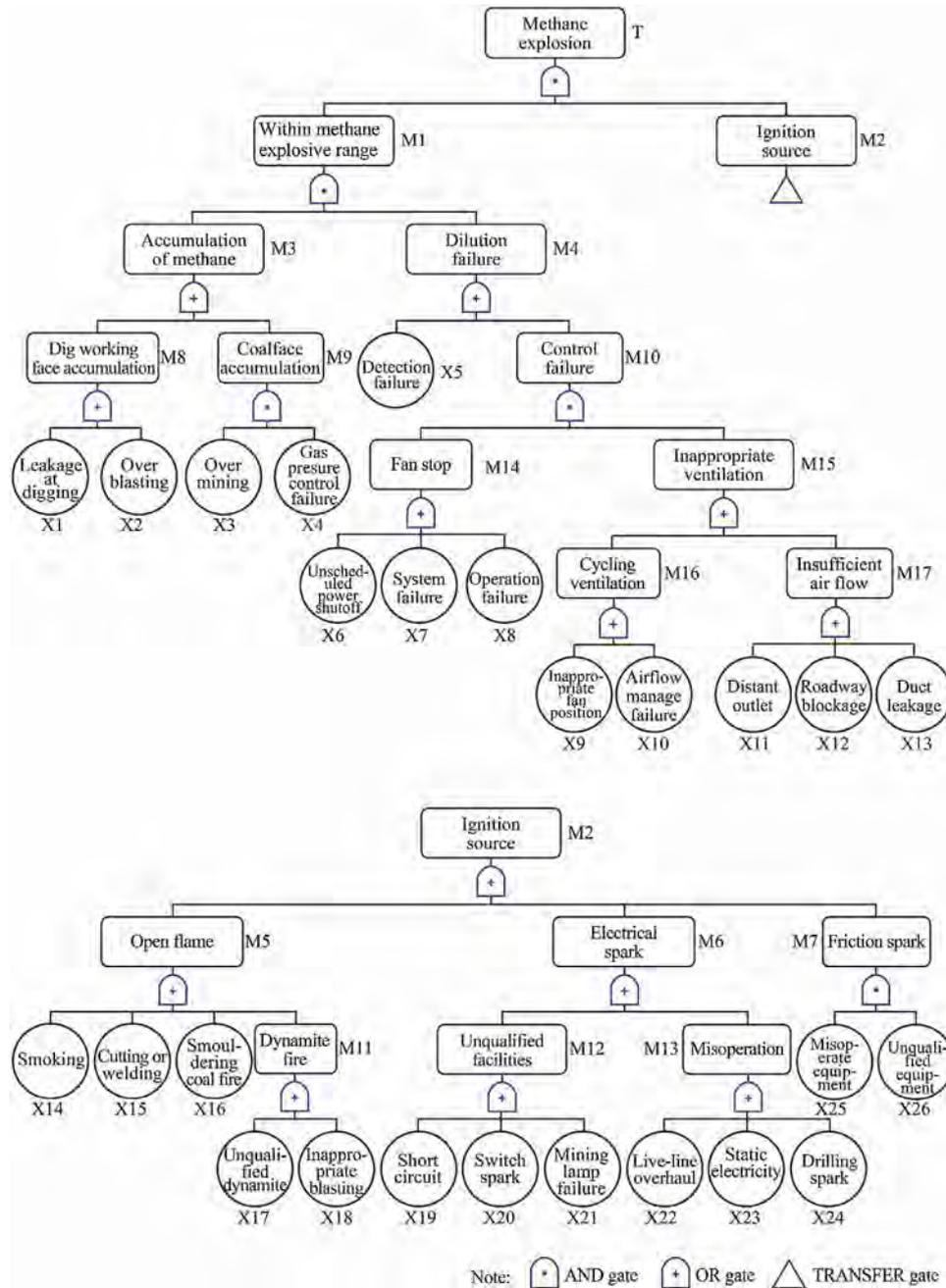
Fig. 2 – Fault tree regarding methane explosion in underground coal mine.
