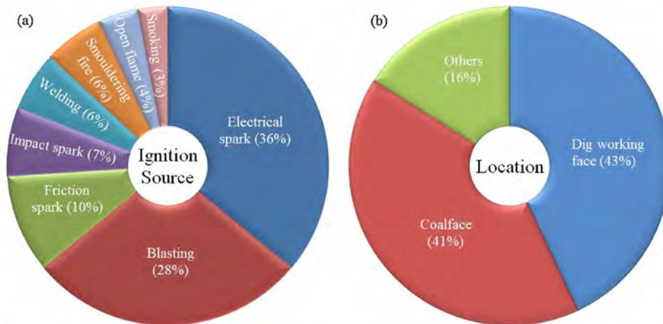
**Fig. 6 – A statistical analysis of coal mine methane burning accidents between 2000 and 2012 in China in the aspect of: (a) ignition source; and (b) location (Xu et al., 2014).**
