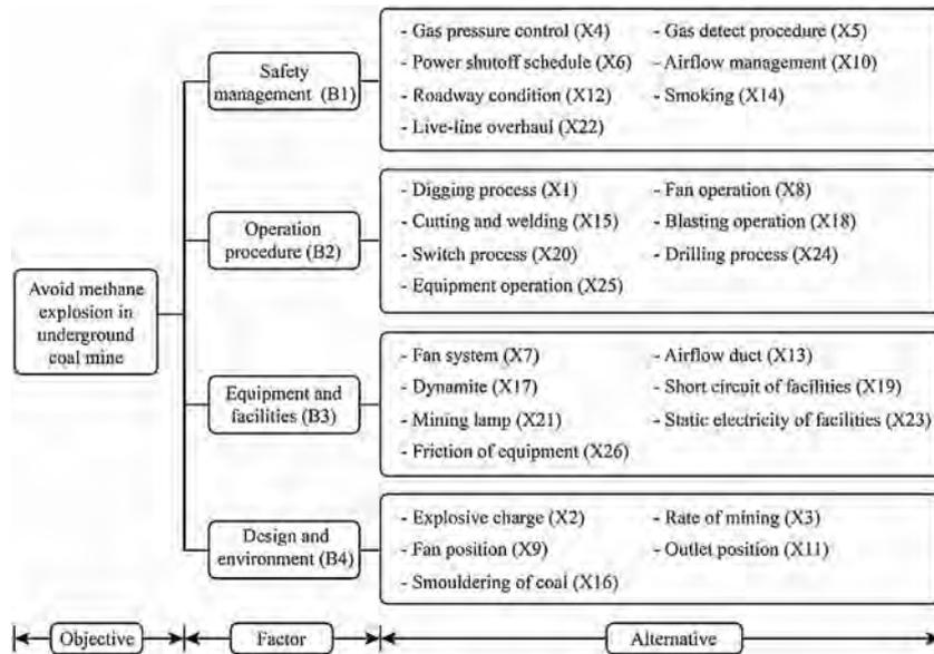
Fig. 3 – AHP model converted from fault tree.
