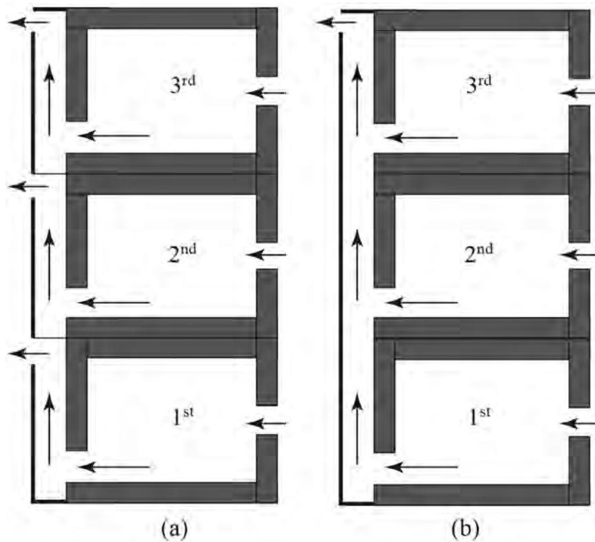
Fig. 2. Two chimney configurations for multi-storey building: (a) separated solar chimney; and (b) combined solar chimney. Figure was revised from Ref. [75].
