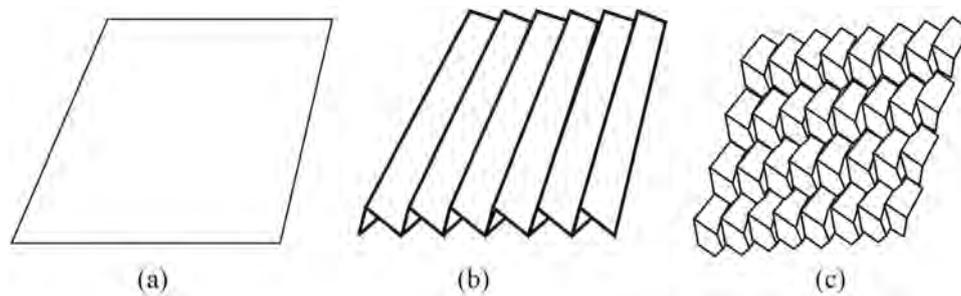
Fig. 5. Three types of solar absorber plates were used for roof solar chimney: (a) flat; (b) V-grooved; and (c) chevron pattern. Figures were revised from Ref. [106].
