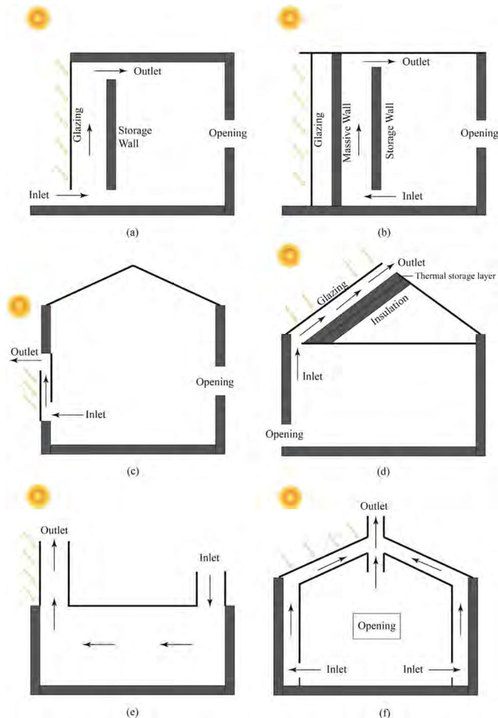
Fig. 1. Typical solar chimneys used in building. Category 1 is the Trombe wall which includes (a), (b), and (c); Category 2 is the roof solar chimney shown in (d) and (e); and Category 3 is the combined solar chimney represented by (f).
