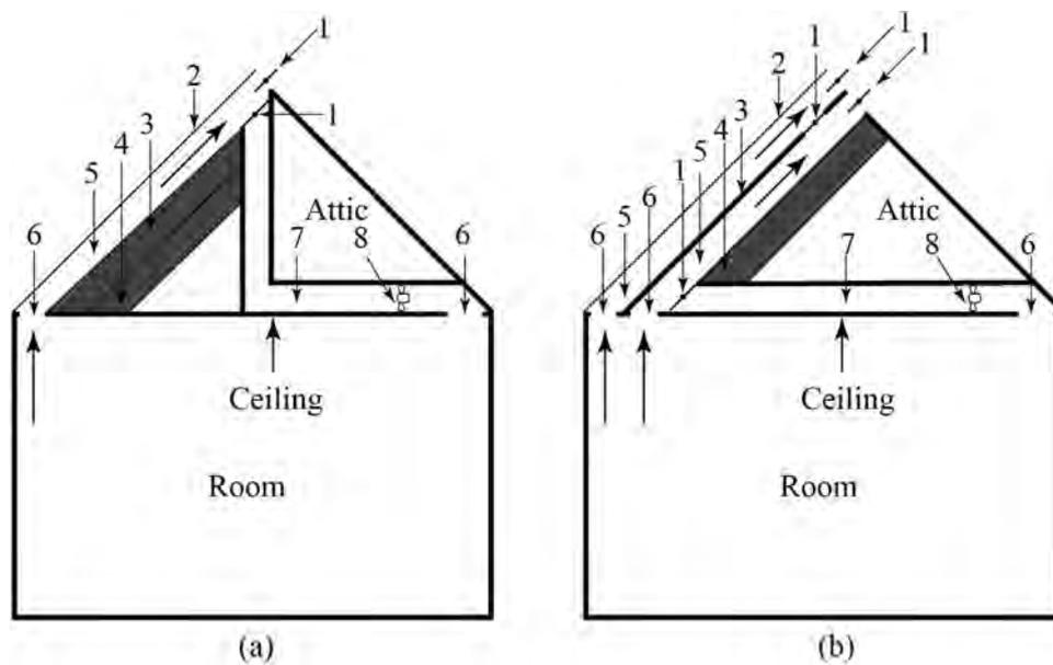
Fig. 6. Structures of single pass (a) and double pass (b) roof solar collector under natural ventilation model: 1 – damper; 2 – glass cover; 3 – absorber plate; 4 – insulation plate; 5 – air channel; 6 – tuyere; 7 – air duct; and 8 – fan. Figures were revised from Ref. [109].
