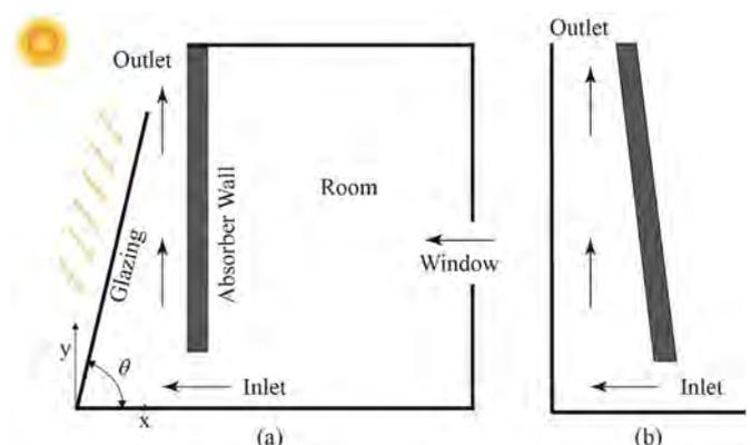
Fig. 4. A schematic of: (a) inclined passive wall solar chimney; and (b) solar chimney with a converging cavity. Figures were revised from Refs. [101,102].
