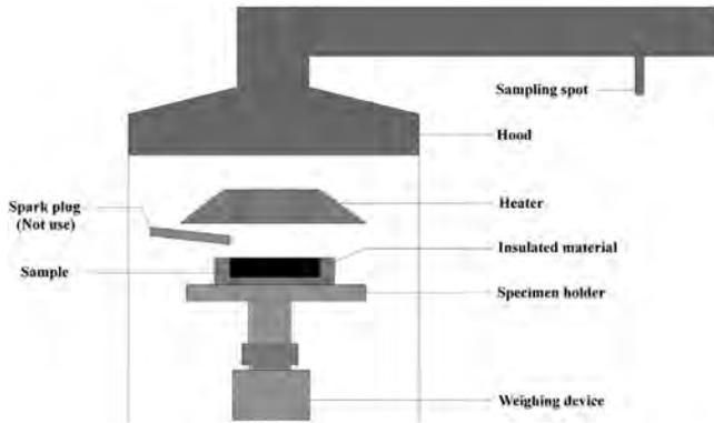
Fig. 1. A view of sample in cone calorimeter.
