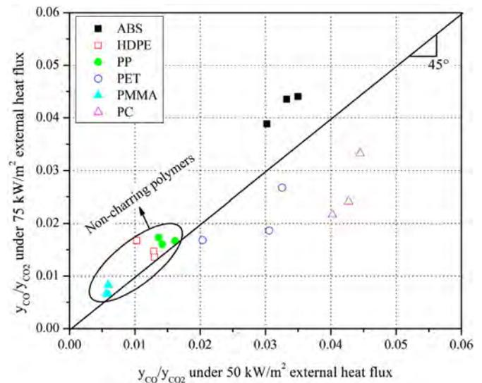
**Fig. 9.** Comparison of  $y_{CO}/y_{CO_2}$  under heat flux.
