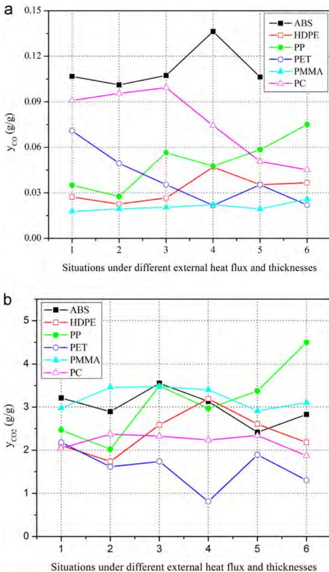
Fig. 10. Comparisons of gas yields under different situations for: (a) CO and (b) CO<sub>2</sub>.
