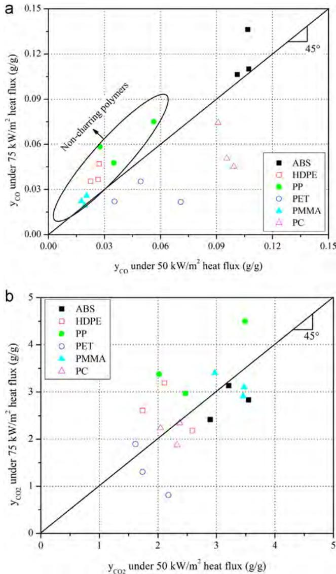
**Fig. 8.** Comparisons of gas yields under 50 and 75 kW/m<sup>2</sup> for (a) CO and (b) CO<sub>2</sub>.
