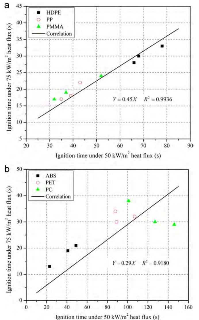
Fig. 4. Influences of external heat flux to autoignition time for: (a) non-charring polymers and (b) charring polymers.
