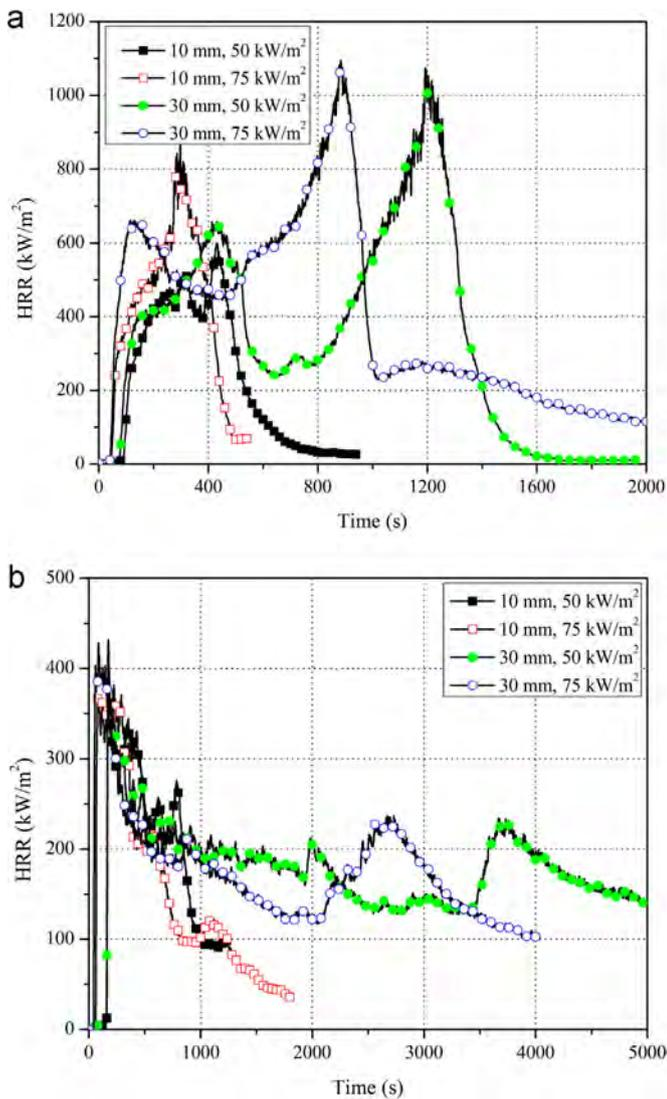
Fig. 5. *HRR* history under external heat flux for: (a) HDPE and (b) PC.
