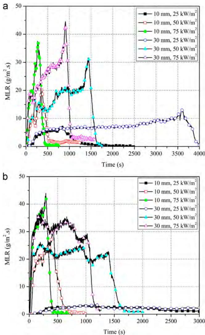
Fig. 6. *MLR* history under external heat flux for (a) PP and (b) ABS.
