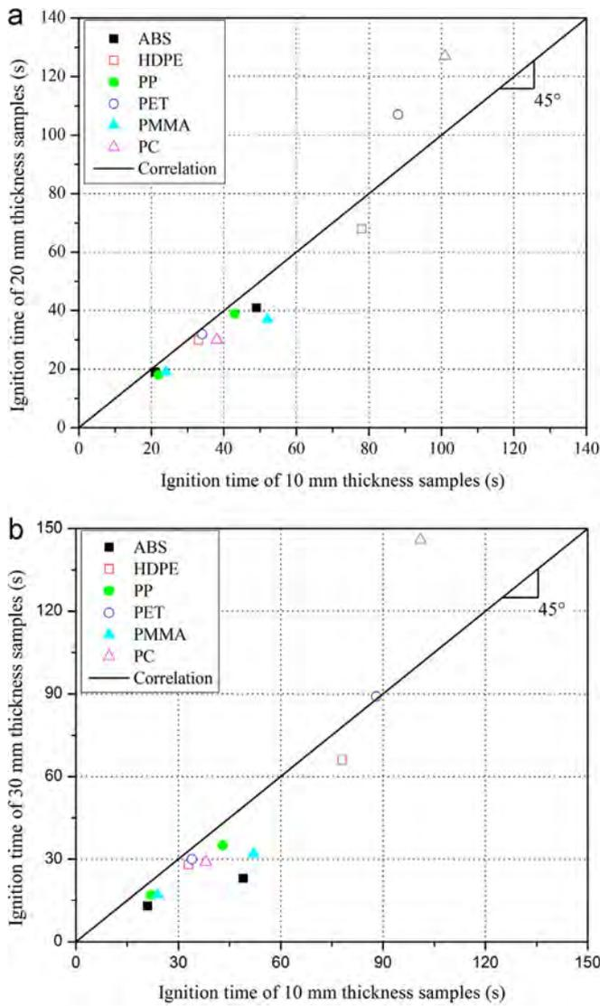
Fig. 2. Comparisons of autoignition time among different sample thicknesses.
