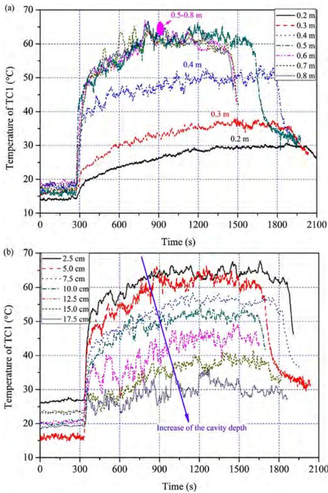
Fig. 9. Temperature near the cavity top (TC1) under the effects of: (a) air inlet height with a cavity depth of 5 cm; and (b) cavity depth with an air inlet height of 0.5 m.
