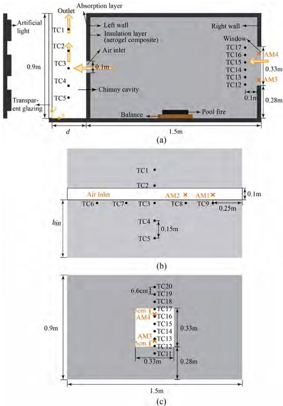
**Fig. 1.** A schematic view of the experimental platform in this study: (a) Experimental setup; (b) measurement spots in the middle plane of chimney cavity ( $x=d/2$ ); and (c) measurement spots 0.1 m from the window ( $x=d+1.4$ ). TC (represented by filled circles) and AM (denoted by crosses) are thermocouple and anemometer, respectively.
