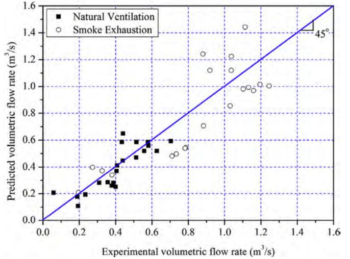
Fig. 13. Validation of the empirical model of this study. The experimental data were converted to full-scale before the comparison.
