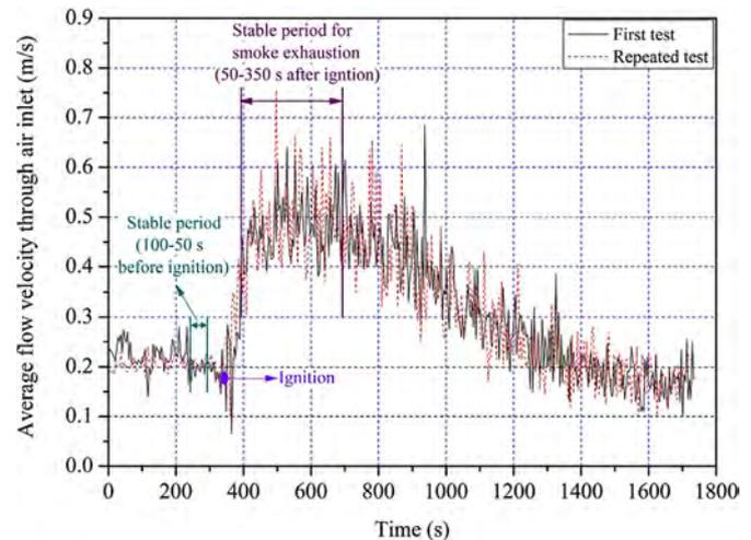
**Fig. 2.** Repeatability of experimental test. The inlet height, cavity depth, solar radiation and fire size are 0.5 m, 10 cm, 800 W/m<sup>2</sup>, and 6.8 kW, respectively.
