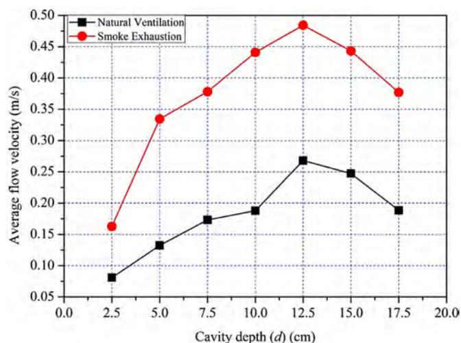
Fig. 8. Influences of cavity depth on natural ventilation and smoke exhaustion for a 0.5 m high air inlet with radiation and fire size are 800 W/m<sup>2</sup> and 6.8 kW, respectively.
