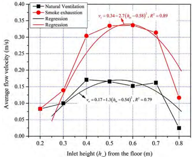
Fig. 7. Influences of inlet height on natural ventilation and smoke exhaustion for a 5 cm cavity depth under a radiation of  $800 \text{ W/m}^2$ . The fire size is 6.8 kW.
