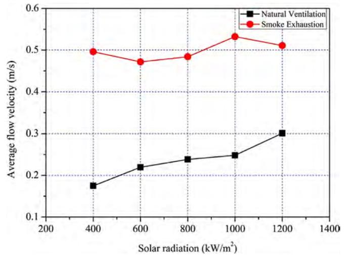
Fig. 10. Influences of solar radiation on natural ventilation and smoke exhaustion.
