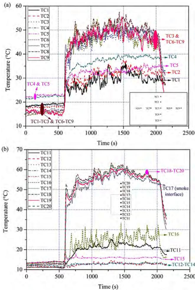
Fig. 6. Temperature histories for locations: (a) inside the chimney cavity; and (b) near the window.
