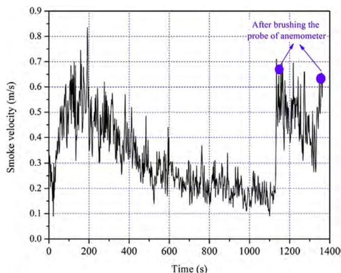
Fig. 3. Measurement of smoke flow velocity after brushing the probe of the anemometer.
