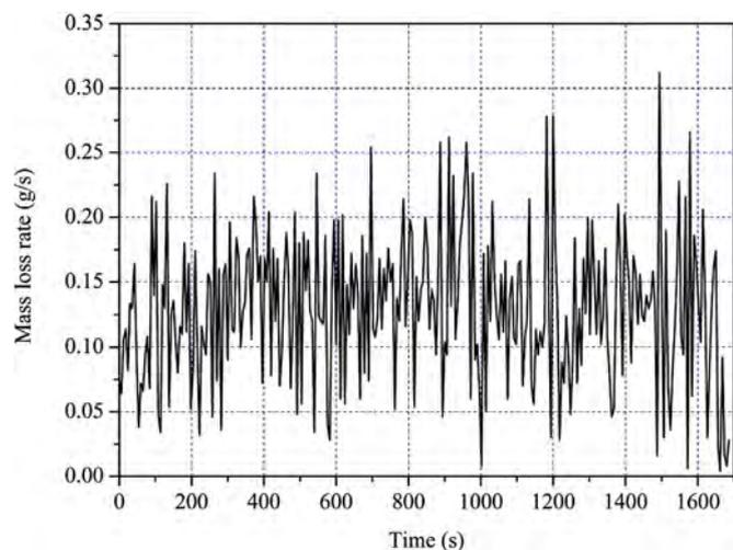
Fig. 4. Mass loss rate history of 12 cm square diesel pool fire with 0.5 m air inlet height and 5 cm cavity depth under  $800 \text{ W/m}^2$  radiation.
