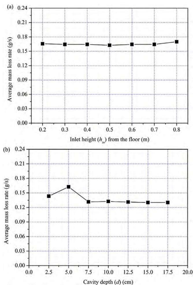
Fig. 5. Average mass loss rate of diesel fire under effects of: (a) inlet height; and (b) cavity depth.
