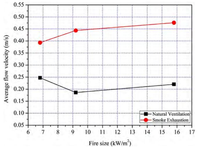
Fig. 11. Influences of fire size on natural ventilation and smoke exhaustion.
