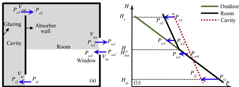
Fig. 4. Solar chimney under fresh-air heating through room (a); and (b) the pressure distributions.
