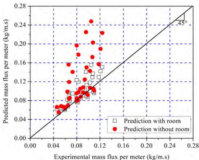
Fig. 8. A comparison between experimental and predicted mass flux per meter. The experimental data come from Ref. [62].
