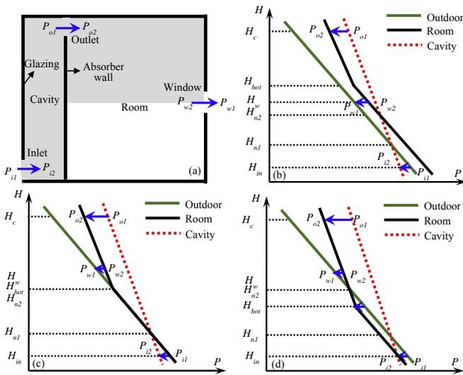
Fig. 3. Solar chimney under fresh-air heating through cavity (a) and pressure distributions under (b) unsteady scenario; (c) steady scenario; and (d) unlikely scenario.
