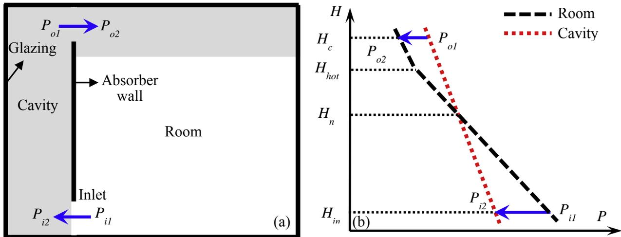
Fig. 5. Solar chimney under sealed heating (a) and the pressure distribution (b) inside chimney cavity and room.
