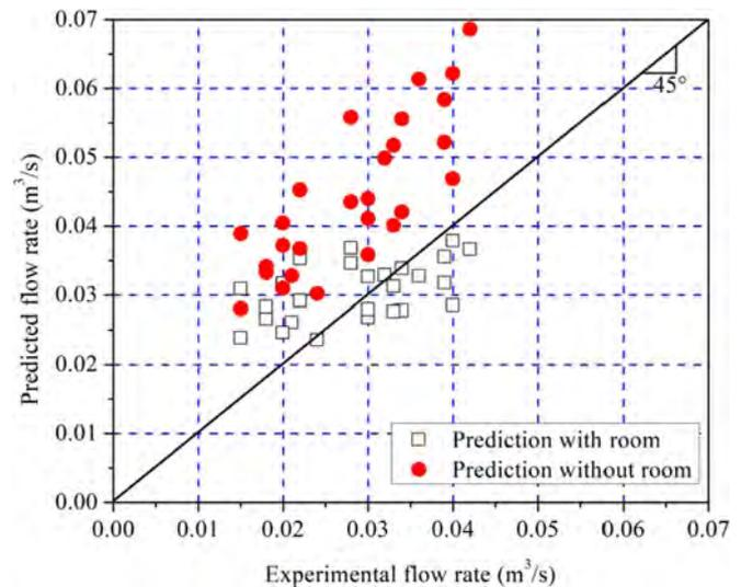
**Fig. 7.** A comparison of experimental and predicted airflow rate through chimney cavity. The experimental data come from Ref. [58].
