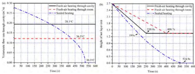
Fig. 9. A comparison of heating performance for three types of solar chimney.
