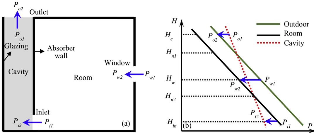
Fig. 2. Solar chimney under fresh-air cooling (a); and pressure distributions in outdoor, room and cavity (b).  $H_{n1}$  and  $H_{n2}$  are the heights of neutral planes in the room and chimney cavity, respectively.
