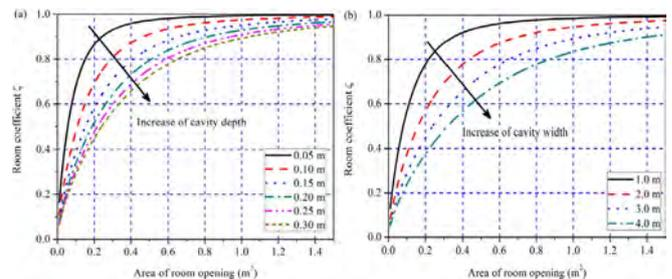
Fig. 6. Relationship between the room coefficient and room opening area for a solar chimney with a 0.3 m high air inlet under various: (a) cavity depths (0.05–0.3 m); and (b) cavity widths (1.0–4.0 m).
