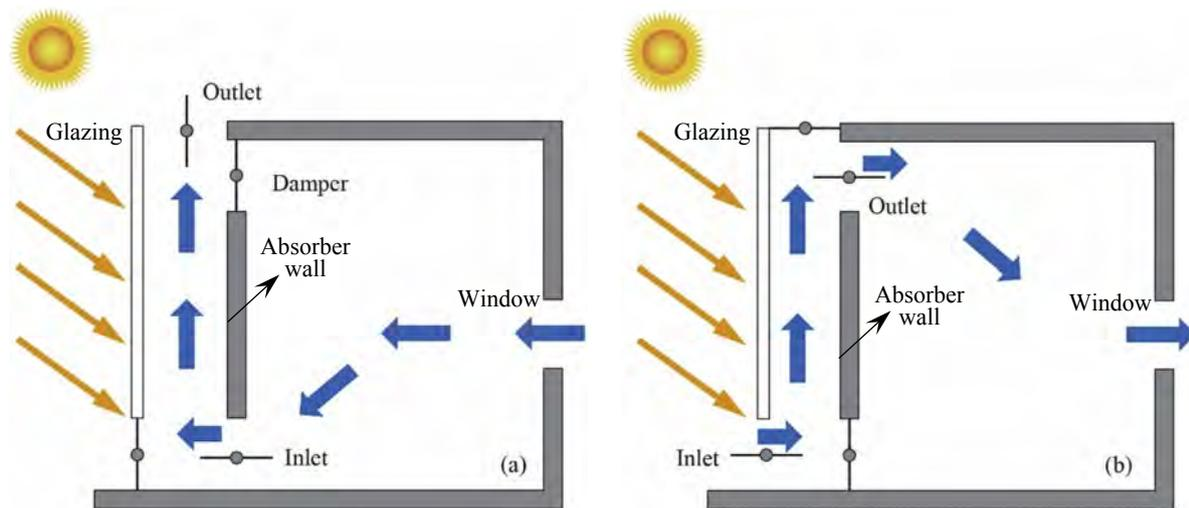
Fig. 1. Typical wall solar chimney under: (a) cooling mode; and (b) heating mode.
